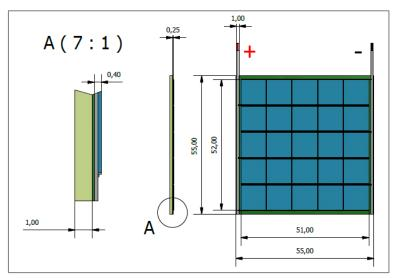
Net Weight: AlN Cell-Array: 12.7g; Al Cell-Array 11.0g
