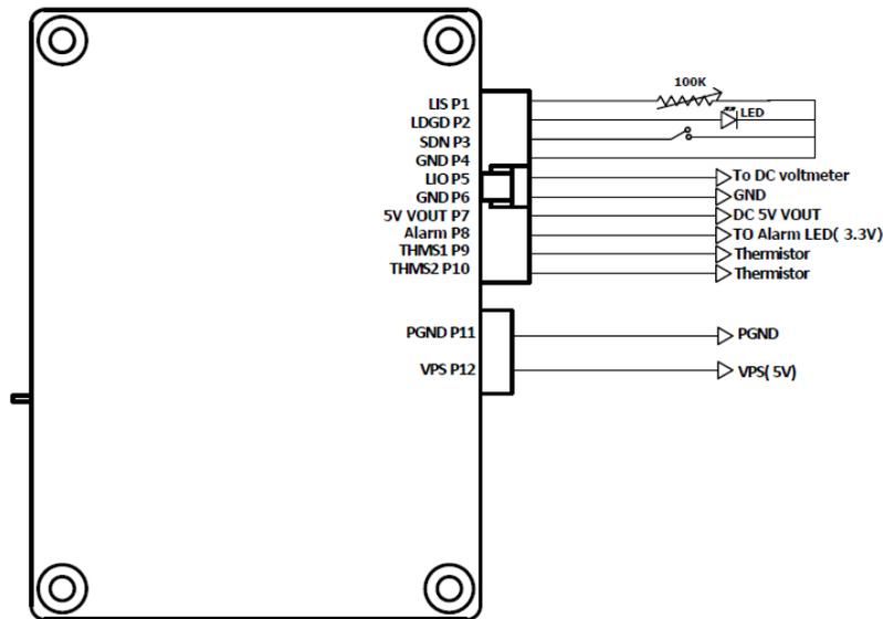
Figure 2. Stand-alone Application Schematic for PPM-010C
